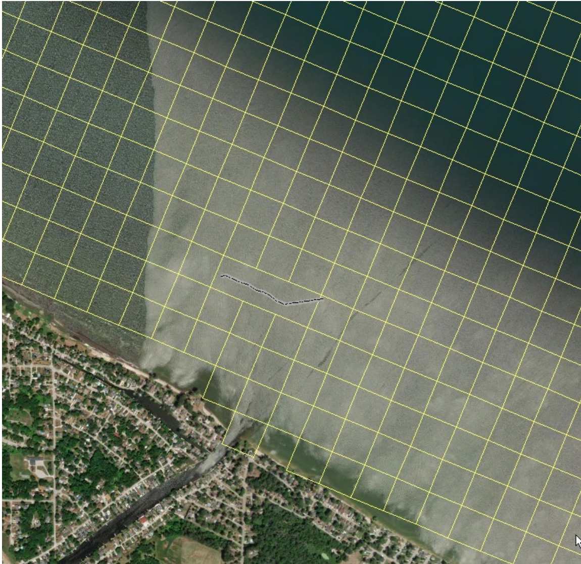
Figure 2-1. Spatial resolution of preliminary feasibility study SWAN model in the vicinity of the reef location (thin black line spanning three model grid cells).
